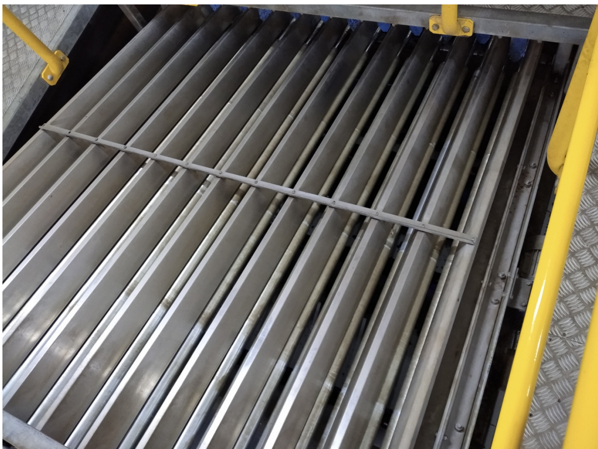
Photo 2: The end of sorting line, where the graded and separated cherries, are put canals of similar size
